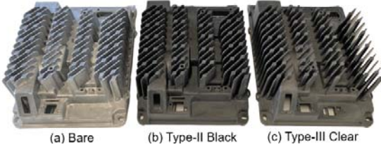
Figure 1. Delta-Q battery charger enclosures, samples made using die-cast process, aluminum A380 alloy; (a) before and after various types of anodization (b) and (c).
